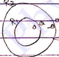
→ 2 spherical concentric shell conductors
